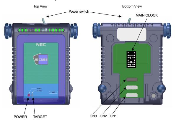
Figure 2-1. Names of Parts of QB-V850EIX3
