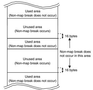
Figure 4-1. Break at Fetching Unused Area
