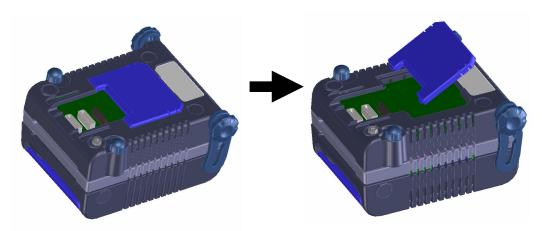
Figure 2-2. Acrylic Board Removal Method
