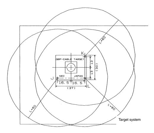
Figure 2-10. Where GND Wire Can Be Connected
