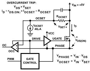
FIGURE 3. OVERCURRENT DETECTION
