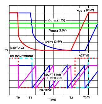
FIGURE 2. OVERCURRENT/UNDERVOLTAGE PROTECTION RESPONSE
