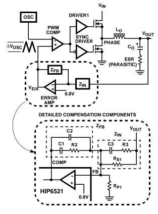
FIGURE 6. VOLTAGE-MODE BUCK CONVERTER COMPENSATION DESIGN
