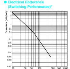
Switching current (A) Must-operate Voltage and Must-release Voltage Distributions
