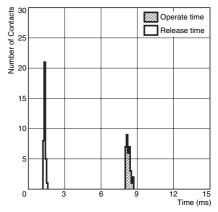
\* The switching performance and interruption performance were measured with a Zener diode and normal diode connected to absorb coil surge. These performance es will be lower if only a normal diode is used.
