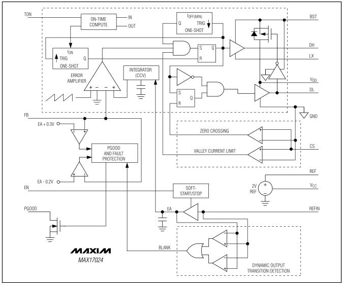
Figure 2. MAX17024 Functional Block Diagram
