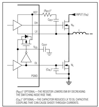
Figure 5. Gate Drive Circuit
