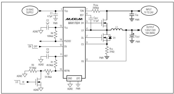
Figure 1. MAX17024 Standard Application Circuit
