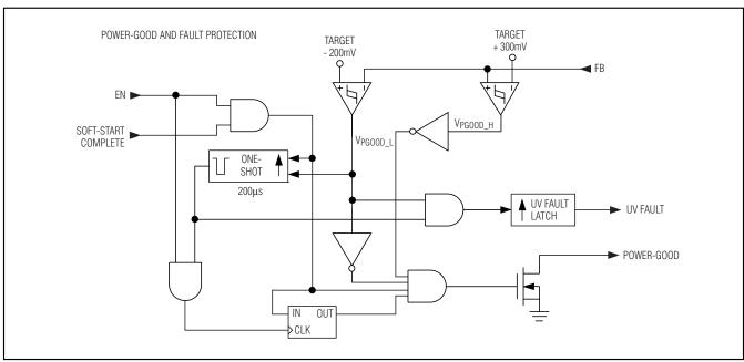
Figure 4. Power-Good and Fault Protection
