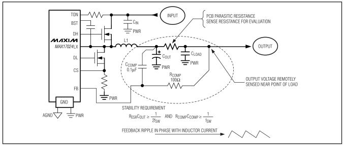
Figure 7. Remote-Sense Compensation for Stability and Noise Immunity
