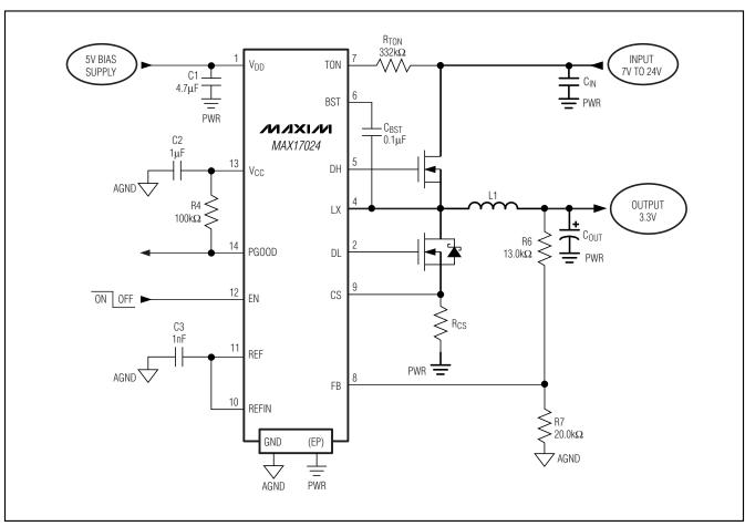
Figure 3. High Output-Voltage Application Using a Feedback Divider
