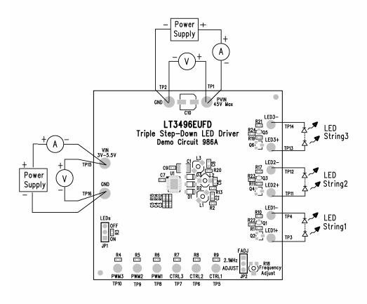
Figure 1. Proper Measurement Equipment Setup
