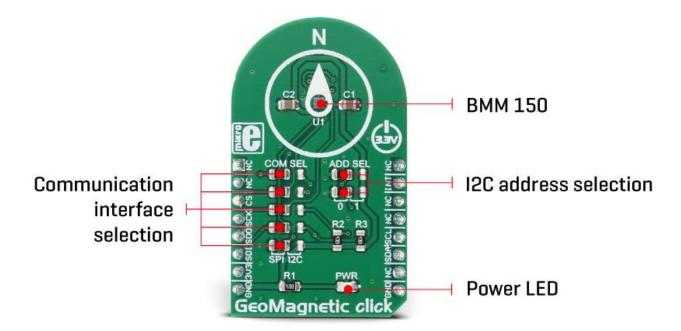
The BMM150 module is able to work in four power modes: Power Off mode, Suspend mode, Sleep mode and Active mode. The overall power consumption is greatly affected by the selection of power modes. All modes except the Power Off mode can be set by programming the appropriate registers. Additionally, while working in Active mode, the power consumption depends on the measurement rate, which can be either timed with the programmed output data rate (Normal mode) or forced by the user (Forced mode).
