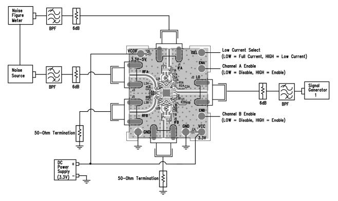
Figure 3. Proper Equipment Setup for Noise Figure Measurement
