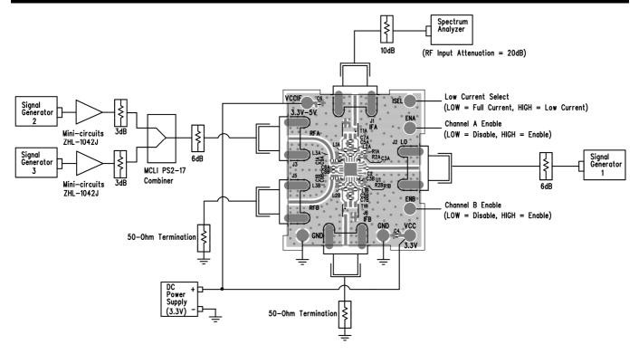
Figure 2. Proper Equipment Setup for RF Performance Measurements
