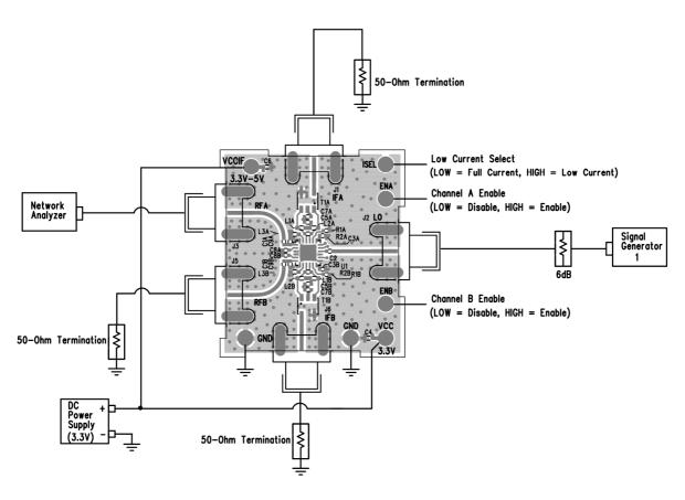
Figure 1. Proper Equipment Setup for Return Loss Measurements
