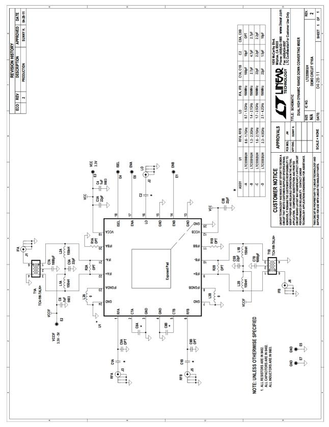
Figure 4. Demonstration Circuit schematic
