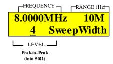
Figure 18: LCD example of displaying sweep width parameter
