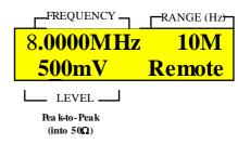
Figure 29: LCD example of sweep start frequency in REMOTE mode
