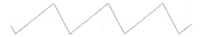
$Example\ of ramp\ wave\ (asymmetric\ triangle), duty\ cycle\ set\ to 100\%.$
