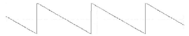
Example of ramp wave (asymmetric triangle), duty cycle set to 20%.
