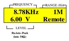
Figure 28: LCD example of displaying frequency when in REMOTE mode
