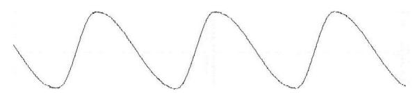
Example of asymmetric sine wave, duty cycle set to 80%.
