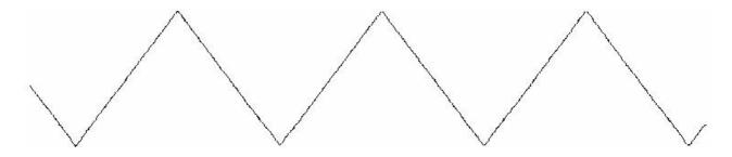
Example of ramp wave (asymmetric triangle), duty cycle set to 70%.
