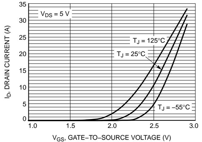
Figure 2. Transfer Characteristics
