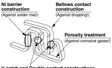
V notch and Double contact constructions (Against foreign particles and flux!)
