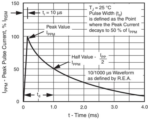
Fig. 3 - Pulse Waveform
