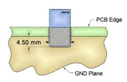
Figure 8 Mounting the module along an edge with overhang. This option is not generally recommended, but is a method to save PCB in an environmentally benign environment
