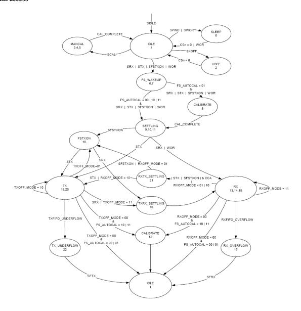
Figure 4 Transceiver state diagram
