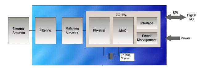
Figure 2 The functionality of the A110LR09C, using an external antenna.
