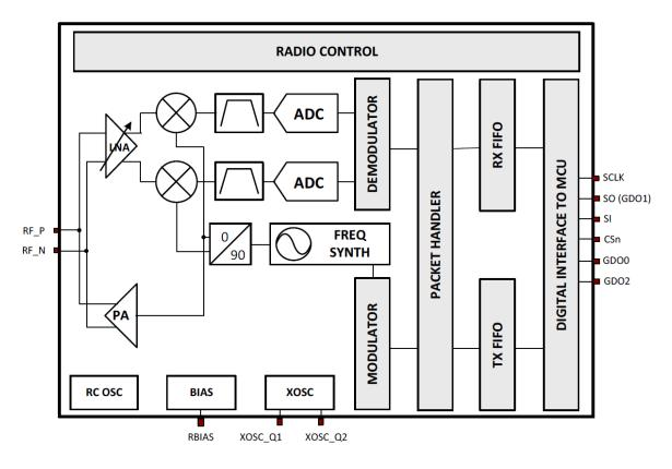
Figure 3 Transceiver IC block diagram.
