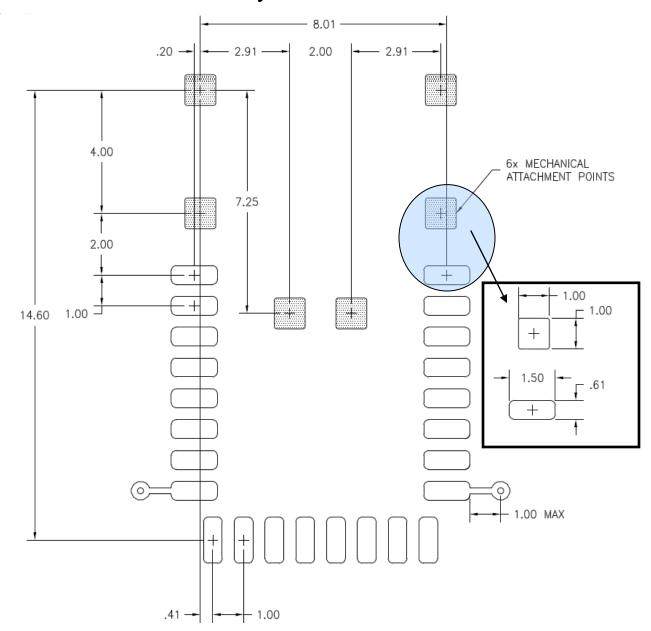
Figure 5 Recommended PCB layout.
