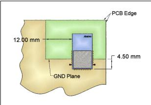
Figure 6 Mounting the module in a corner
