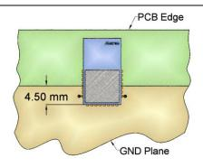
Figure 7 Mounting the module along an edge
