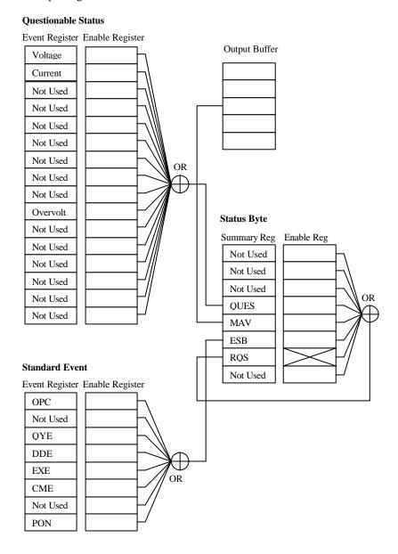
**Event Register** is a read only register. Bits in an event register are set depending on the state of the power supply.
