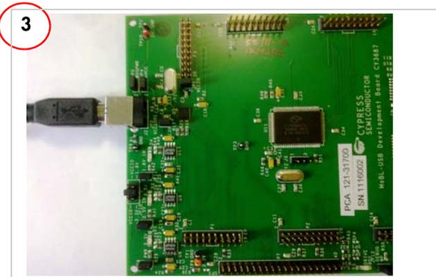
3 Connect a USB A-to-B cable between the development board J2 connector and USB Host port on a Windows PC. Windows Hardware wizard window pops up at this moment. Follow the steps (5-10) outlined in section 6.2.1 of Kit User Guide. Point the Windows Hardware Wizard to the directory of the relevant USB driver for Windows OS platform to which the MOBL-USB FX2LP18 development board is connected.
