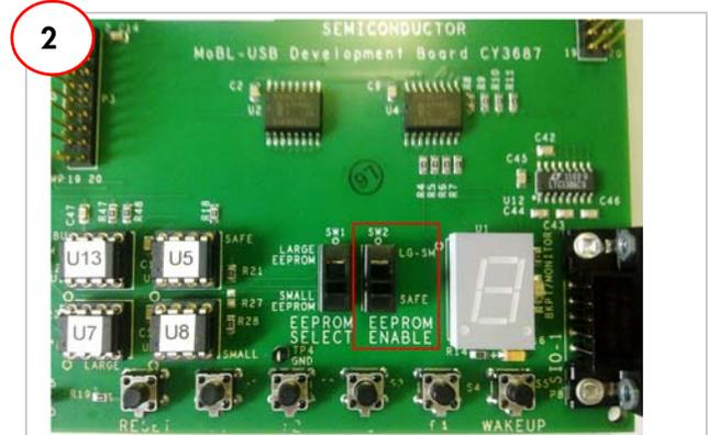
2 Set the switch SW2 in 'SAFE' mode as shown above.
