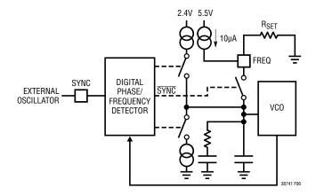
Figure 6. Phase-Locked Loop Block Diagram
