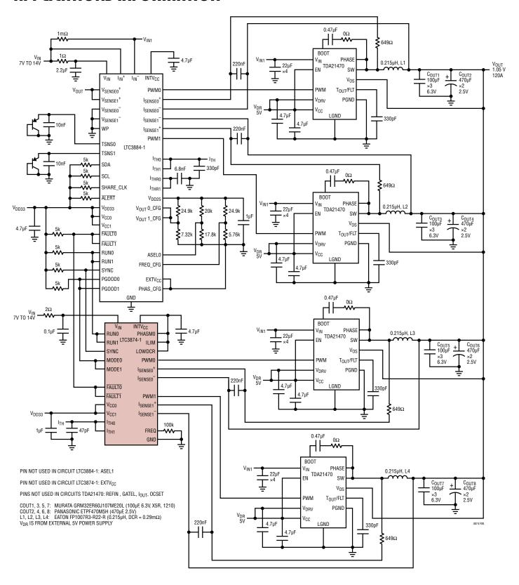
Figure 8. High Efficiency 500kHz 4-Phase 1.05V Step-Down Converter
