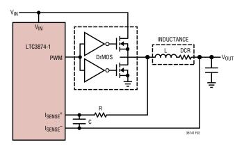
**Figure 2 Inductor DCR Current Sensing**
