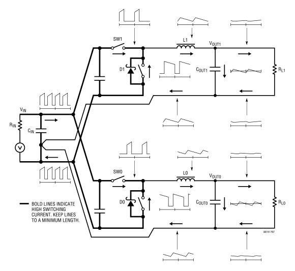
Figure 7. Recommended Printed Circuit Layout Diagram
