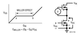
Figure 3. Gate Charge Characteristic
