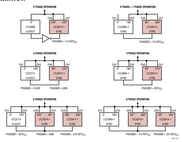
Figure 1. Multiphase Operation
