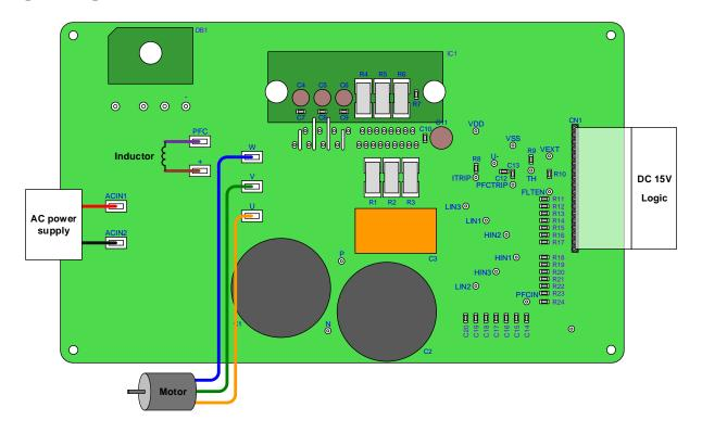
**Step1**: Connect IPM, the three power supplies, logic parts, inductor and the motor to the evaluation board, and confirm that each power supply is OFF at this time.
