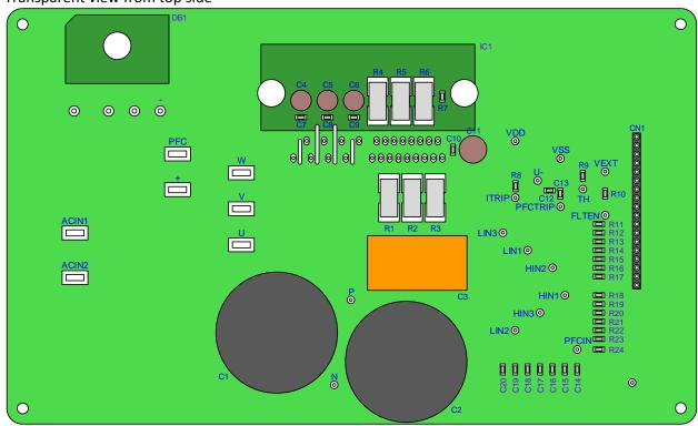
\* IC1, DB1, R11-24, C14-20 are arranged on solder side.
