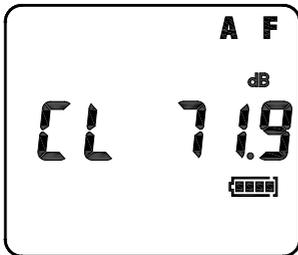
6. Adjust the meter's potentiometer (recessed at top of meter) using the supplied adjustment tool until the display reads 114db, matching the 114db output level of the calibrator.
