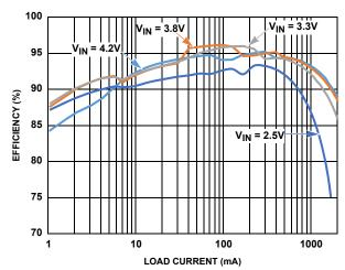
FIGURE 2. EFFICIENCY vs OUTPUT CURRENT (VOUT = 3.3V)
