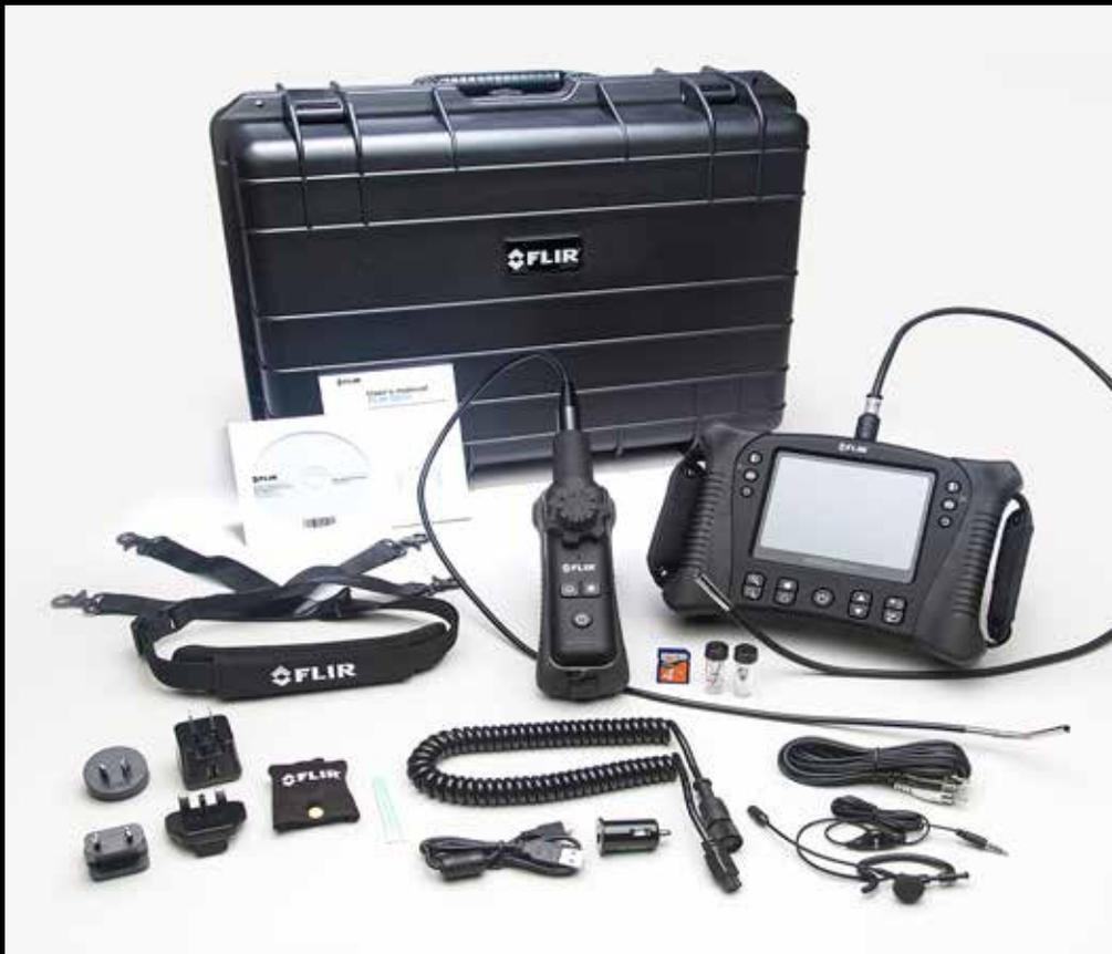
FLIR VS70-Kit-W Wireless bundle includes the base kit plus 8mm long-focus (3.15"/8cm) camera on a 1-meter semi-rigid cable, wireless handset with dedicated 6mm camera with 2-way (240°) articulation on a 1-meter semi-rigid cable.
