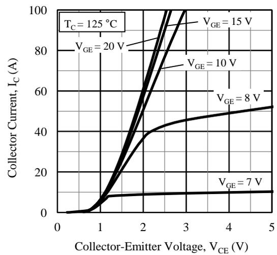
Figure 6. Output Characteristics ( $T_C = 125\text{ }^\circ\text{C}$ )
