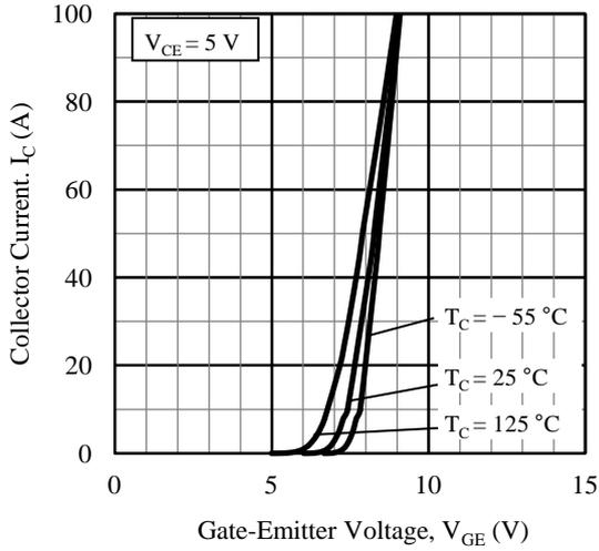
Figure 7. Transfer Characteristics
