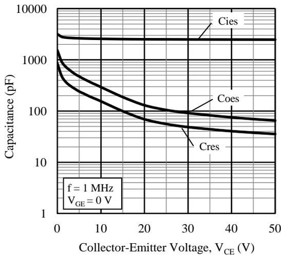
Figure 11. Capacitance Characteristics
