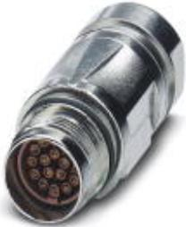
Coupler connector, straight, SPEEDCON locking, M17, Number of positions: 8, Type of contact: Socket, Crimp connection, shielded: yes, Cable diameter: 8 mm...10 mm
