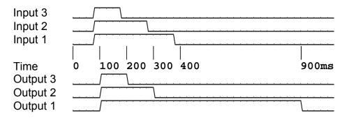
The second diagram shows the same operation at the transmitter, but with the receiver configured with a 20ms hang time.
