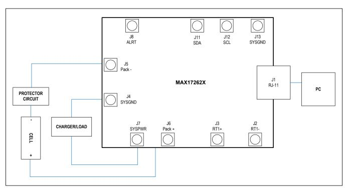
Figure 1. MAX17262 Board Connections
