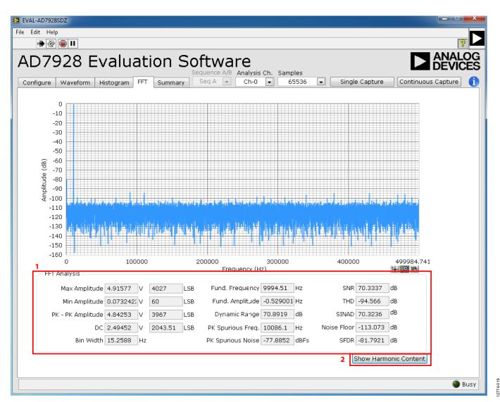
Figure 20. **FFT** Capture Tab
