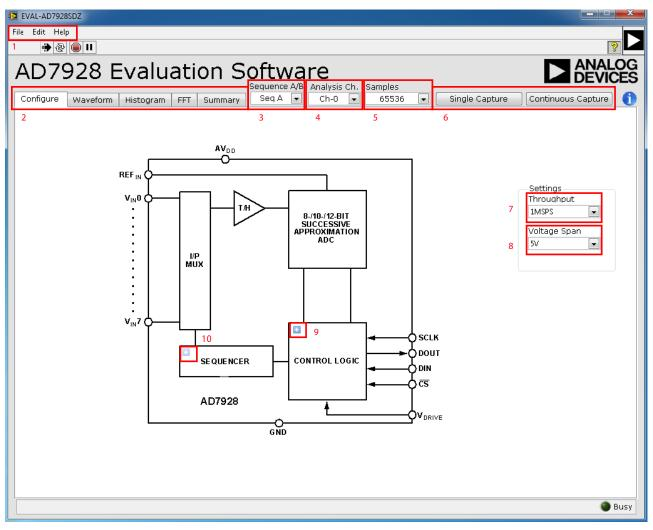
Figure 13. AD7928 Evaluation Software Main Window
