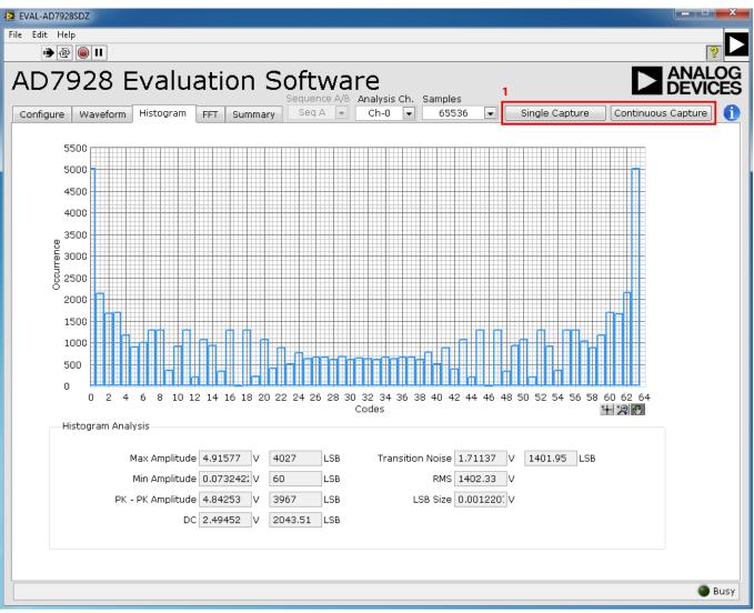
Figure 19. Histogram Capture Tab
