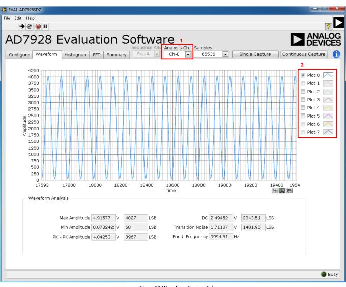
Figure 18. Waveform Capture Tab
