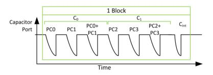
Figure 3-3 Charging-/ discharging cycles floating, compensated, single and differential sensors Figure 3-3 shows a CDC example with one floating single sensor plus reference / one floating differential sensor. One measurement block is made of 3 discharge time measurements for each capacitor, including the external compensation measurement, and an additional one for measuring the internal stray capacitances and comparator delay. See section 3.6 for further details on the compensation.
