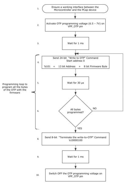
sequence of steps to be performed to program the firmware into the OTP:
