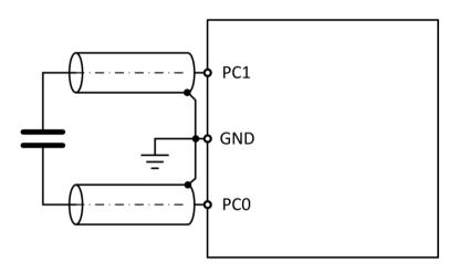
Figure 3-11 shows how shielded cables should be connected for compensation of the external parasitic capacitances.
