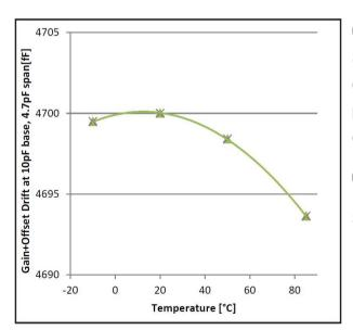
Figure 2-7 Gain Drift vs. Temperature
