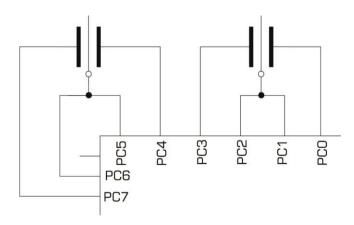
Figure 3-8: Differential sensors, floating
