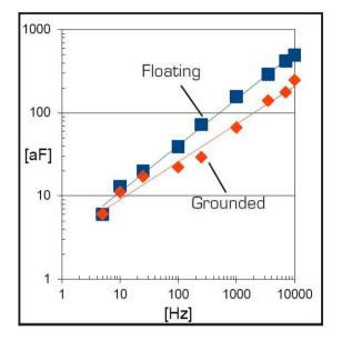
Figure 2-1 Typical Capacitive Noise vs. Output Data Rate, with 10 pF Base Capacitance, V = 3.0 V  $\,$
