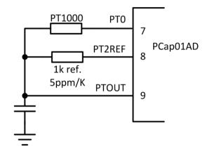
Figure 3-14 RDC with external resistors
