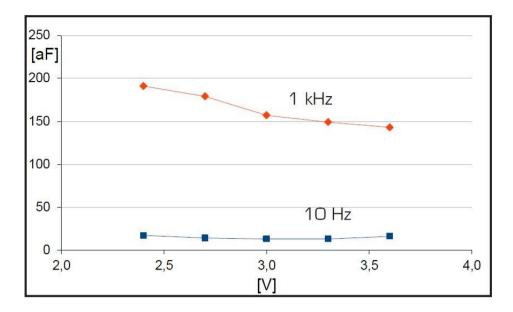
Figure 2-4 RMS Noise vs. Supply Voltage
