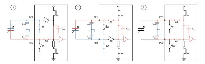
Figure 3-12 Floating capacitors, external compensation measurements, the three measurements that are made for each floating capacitor.
