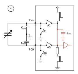
Figure 3-13 Grounded/floating capacitors, internal compensation measurement
