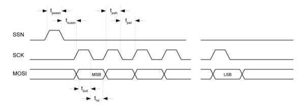
Figure 4-4: SPI Write
