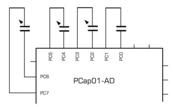
Figure 3-6: Single sensors, floating, up to 3 sensors (C1 to C3) and one reference (CO)
