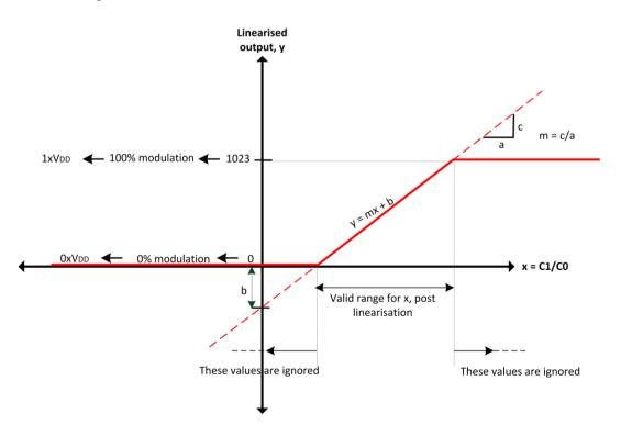
Figure 4-8: PWM-PDM linearization
