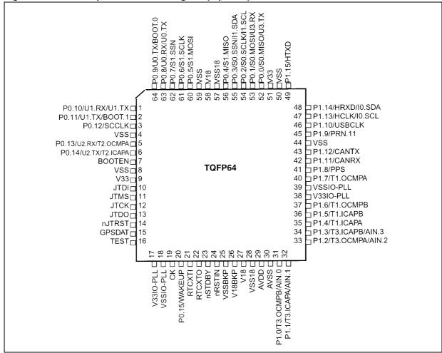
Figure 3. LQFP64 pin connection diagram (top view)
