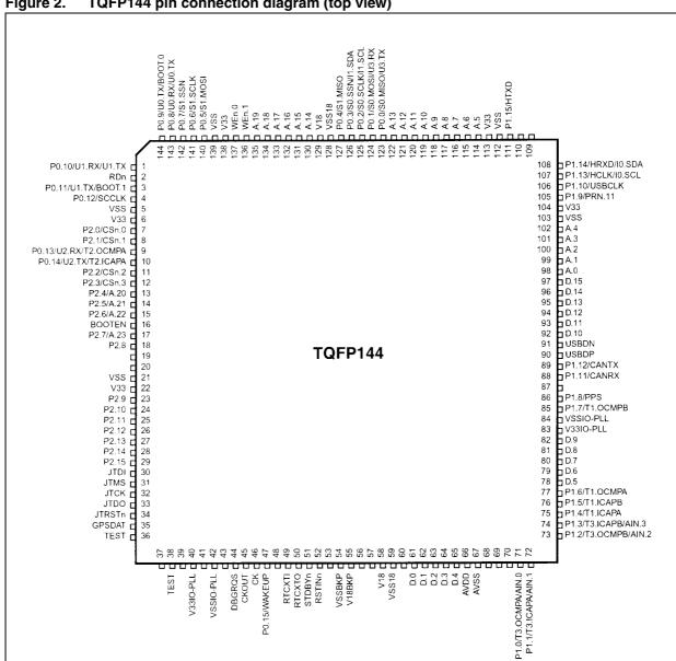
Figure 2. TQFP144 pin connection diagram (top view)
