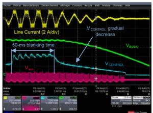
b) Start of operation when V<sub>in,rms</sub> exceeds (V<sub>in,rms</sub>)<sub>BOH</sub> (NCP1612A)
