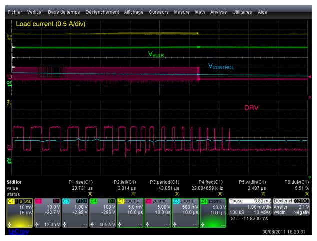
Figure 16. Soft Over-Voltage Protection
