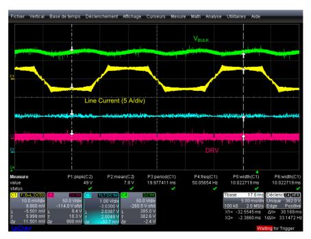
Figure 14. Over-Current Situation (85 V, 0.5 A Load Current)
