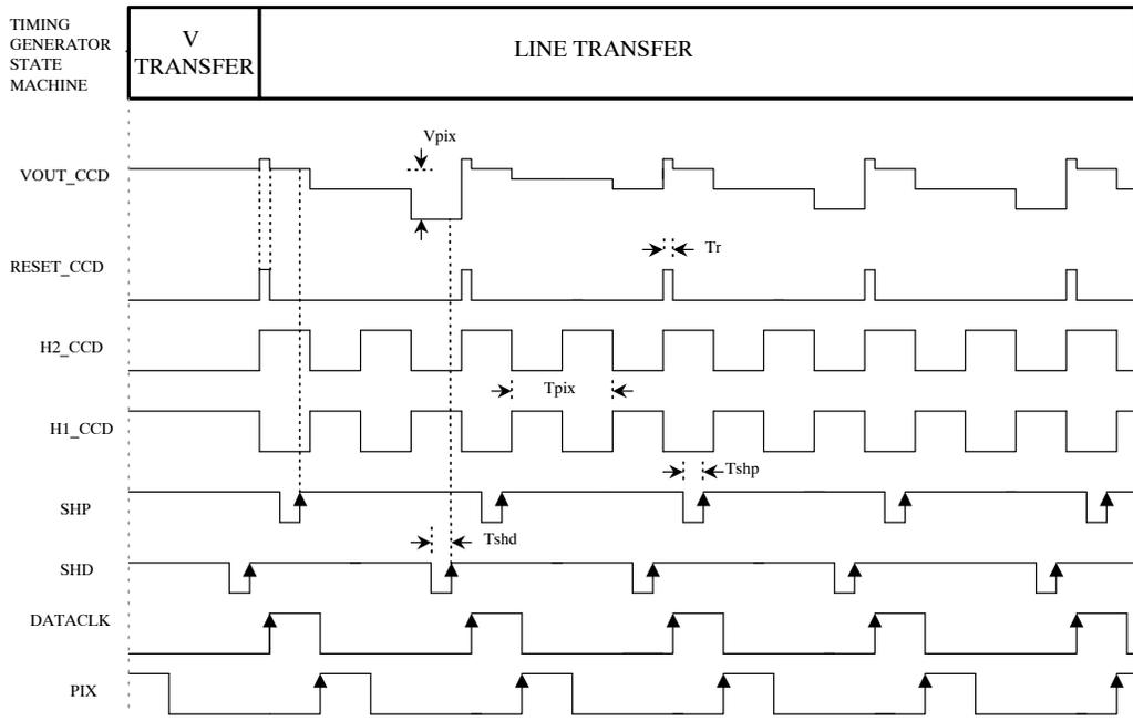
Figure 10. Horizontal Timing – 2x2 Binning Mode Line Transfer
