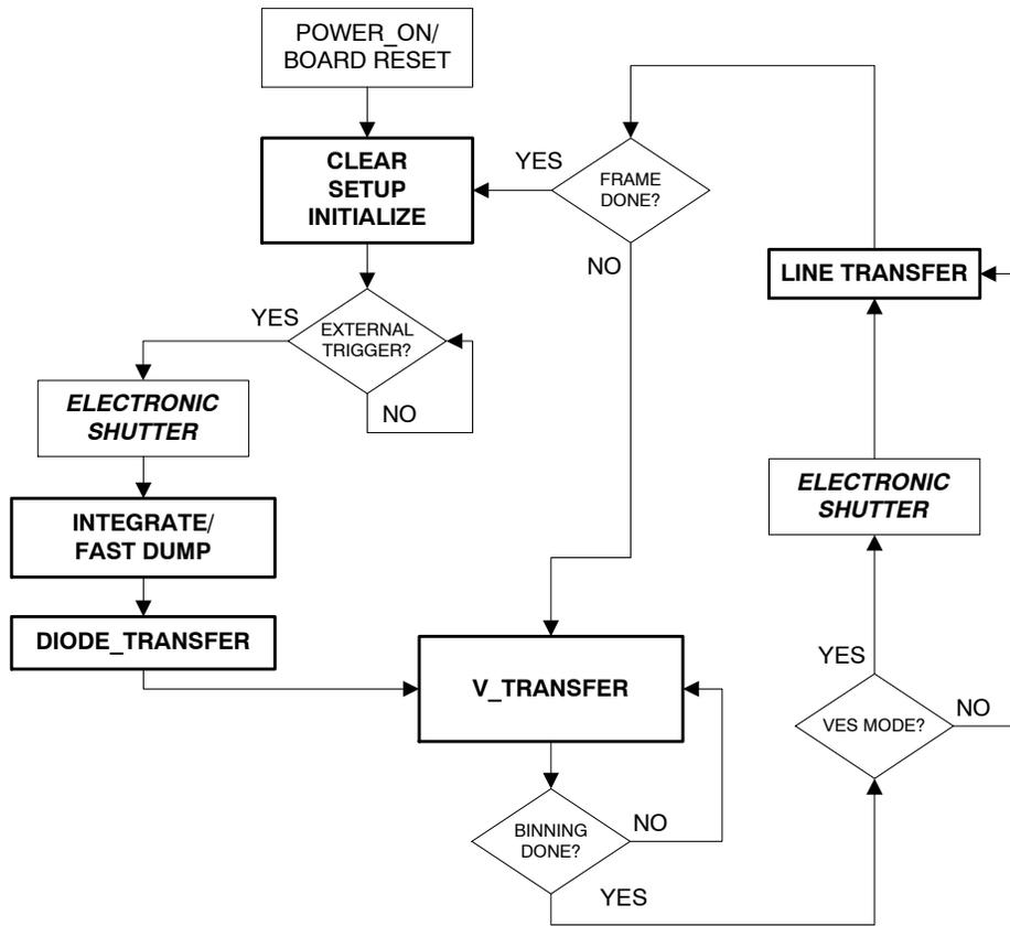
Figure 3. Timing Generator State Machine (Single Capture Mode)
