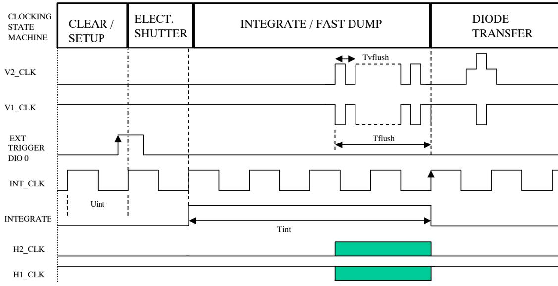
Figure 11. Single Capture with External Trigger Timing
