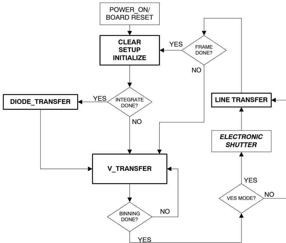
Figure 2. Timing Generator State Machine (Free-Running Mode)
