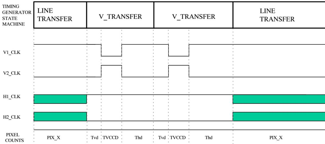
**Figure 7. Vertical Transfer Timing – 2x2 Binning Mode**
