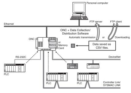
Example: Data collected using the Data Collection/ Distribution Software can be displayed in Excel as shown below. A sample CSV file is shown set to collect data when bit 00 in CIO 0000 turns ON.
