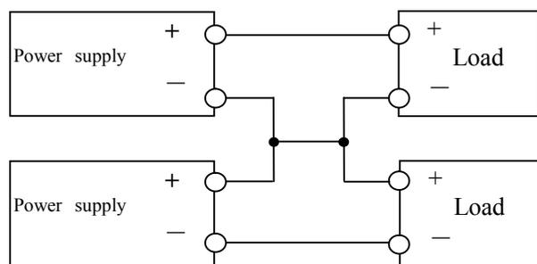
(Note1) Please connect a diode for by-pass when using method (A) of the series operation.
