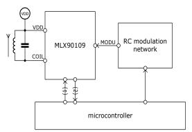
(1): MODE/SPEED config settings (2): DATA/CLOCK outputs
