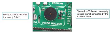
Figure 14-1: Piezo Buzzer
