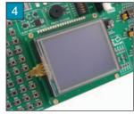
Figure 19-1: Placing touch panel over a GLCD
