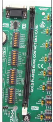
Figure 2-1: DIMM-168P connector
