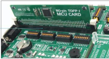
Figure 2-2: DIMM-168P connector with the MCU card inserted
