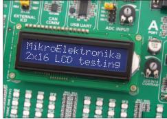
Figure 17-2: Alphanumeric 2x16 LCD
