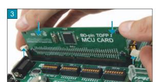
Push the MCU card down gently into the DIMM-168P connector and lift extraction levers slowly at the same time
