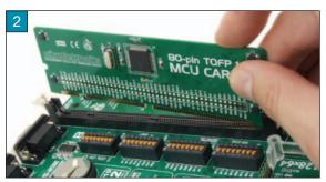
Place the MCU card into the DIMM-168P connector
