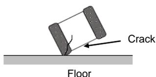
3. When printed circuit boards are piled up or handled, the corners of another printed circuit board should not be allowed to hit the capacitor in order to avoid a crack or other damage to the capacitor.
