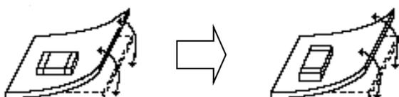
Locate chip horizontal to the direction in which stress acts
