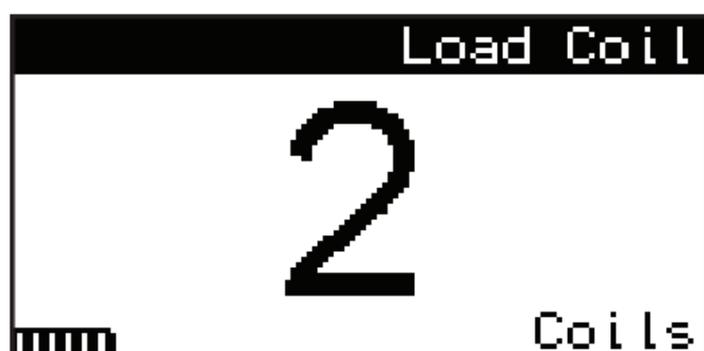
Until a reading is in progress “-” is displayed. When it is done, a number from 0 to >5 will be displayed.
