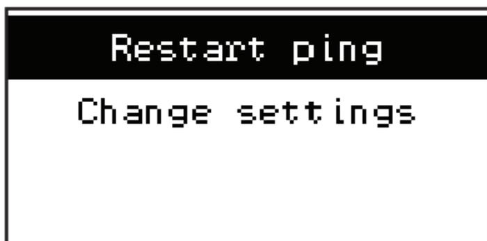
Type in the IP address of the destination you wish to ping. Press **ENTER**, and then move the cursor to “Restart ping” and press **ENTER** to start the ping. The first example shows no response and the second example shows successful ping.
