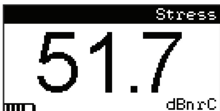
3. Stressed noise level reading will now be indicated on the LCD. When performing the Stress test on complete end-to-end circuits, use the following noise metallic readings (as a guide) to determine pair quality.
