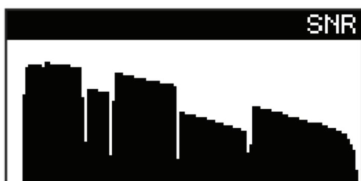
Signal-to-noise histograms show SNR for each of the xDSL frequency bands for the selected profile.
