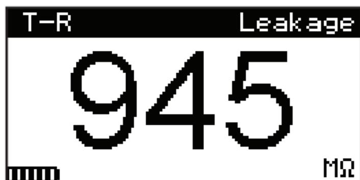
4. For best results, leave the polarity in either direction for at least 15 seconds. Then change it again and continue to check the readings. A sudden drop in the resistance, or readings that waver, are a sign of galvanic corrosion break down. Also the Tip-to-Ground and Ring-to-Ground measurement must be rechecked for any change after the polarity reversal.
