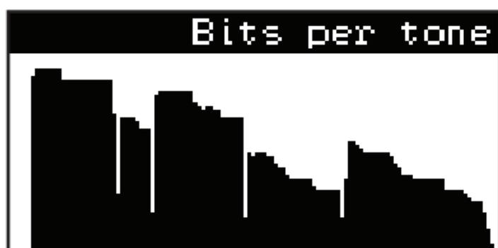
The Bits per tone histogram shows number of allocated bits per each of the xDSL frequency bands for the selected profile.
