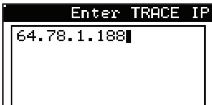
Type the IP address you wish to trace and press **ENTER**. Then move the cursor to “Restart traceroute” and press **ENTER** to start the Trace.
