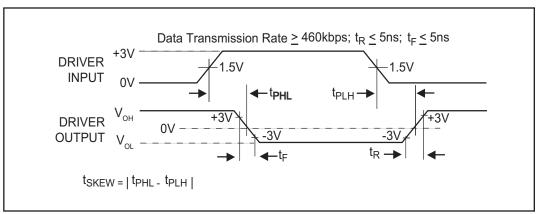
Figure 5. Driver Propagation Delay
