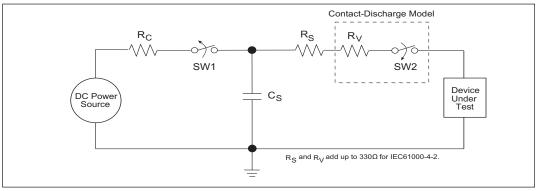
Figure 11. ESD Test Circuit for IEC61000-4-2
