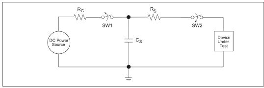
Figure 10. ESD Test Circuit for Human Body Model
