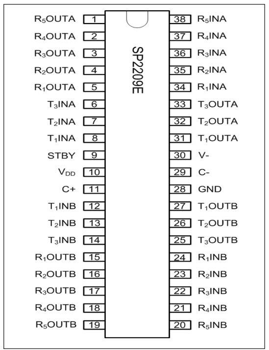
Figure 1. Pinout Configuration for the SP2209E
