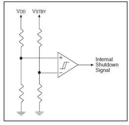
Figure 9 Internal Standby Detection Circuit
