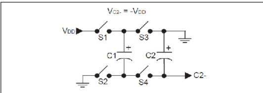
Figure 7. Charge Pump Circuit
