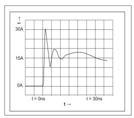
Figure 12. ESD Test Waveform for IEC61000-4-2
