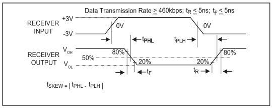
Figure 6. Receiver Propagation Delay
