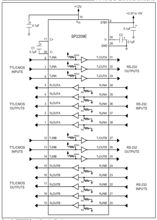
Figure 2. SP2209E Typical Operating Circuits
