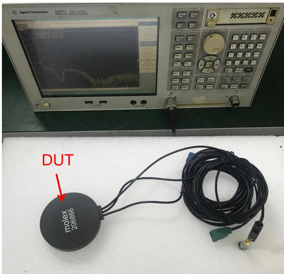
FIGURE4.1.1 ANTENNA TESTED WITH VNA E5071C
