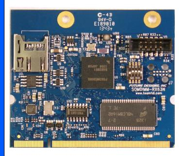
Modular RX63N based Microcontroller Plug-In System-On-Module
