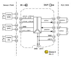
Figure 1 Block diagram with connection terminal blocks
