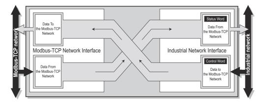
Each data buffer holds a maximum of 256 bytes of data, and the total amount of data that can be exchanged at any time cannot exceed 512 bytes. The first two I/O mapped bytes in either direction can be dedicated for control/status information, and another eight bytes of data coming from the Modbus-TCP network can feature a live list.
