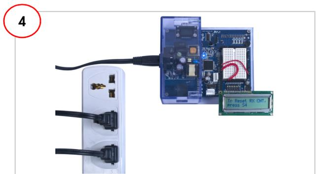
1. Connect the LCD Module to LCD1 header.
