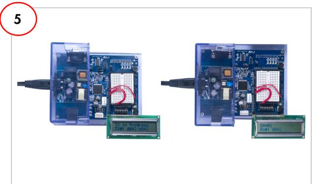
1. Push the reset button S2 on both nodes. A message "PLC Demo" initially appears on the LCD. The kit will be a transmitter if the DIP switch connected to PO[7] is pulled high, else the kit will act as a receiver.
