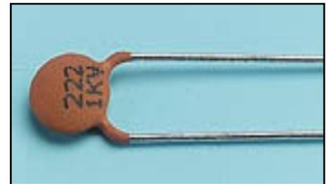
Example:  $104 = 10 + 0000$  (4 zero's) = **100,000 pF** (which is also  $0.1\ \mu\text{F}$ )
