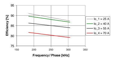
III 3- and 4-Phase Converter: Efficiency vs. Load current
