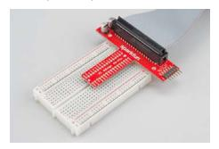
The Pi Wedge in a breadboard
