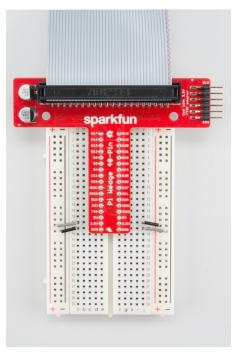
Jumpering power to the breadboard rails
