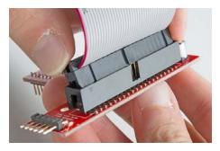
Inserting the ribbon cable
