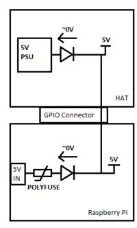
The first recommendation is to duplicate the fuse and MOSFET + BJT power protection circuit as seen on the Pi itself. This circuit is a variant on the "ideal diode" circuit.
