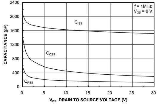
Figure 8. Capacitance Characteristics.
