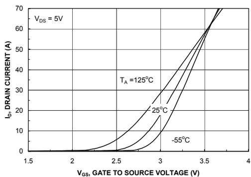
Figure 5. Transfer Characteristics.
