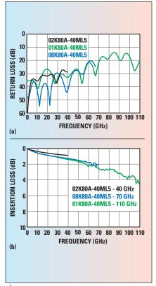
▲ Fig. 4 Measured reflection loss of solderless PCB mount connectors (a) and measured insertion loss (b).
