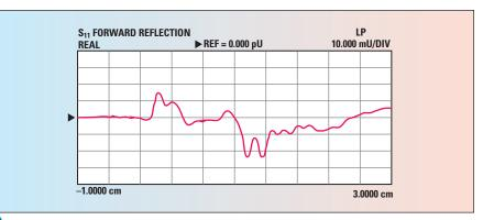
**A** Fig. 5 Gated  $S_{11}$  in TD of the 110 GHz connectors 01K80A-40ML5.
