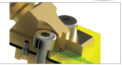
Fig. 3 Detailed view of the PCB contact area with cut-out.
