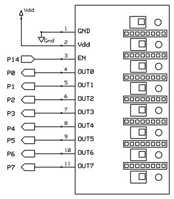
Figure 1: Infrared Line Follower Quick-Start Circuit
