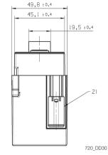
Permitted torque 6Nm max. One-time mounting only, no recurring screw fastening permitted.
