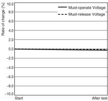
Characteristics were measured after applying a shock of 490 m/s² to the test piece 3 times each in 6 directions along 3 axes. The percentage rate of change is the average value for all of the samples.
