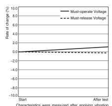
Characteristics were measured after applying vibration at a frequency of 5 to 200 to 5 Hz, acceleration of 44.1 m/s² to the test piece (not energized) for 2 hours each in 3 directions. The percentage rate of change is the average value for all of the samples.
