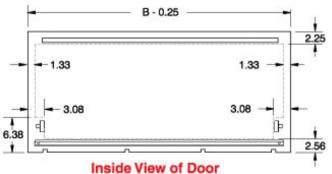
Clearance area for mounting hardware on
