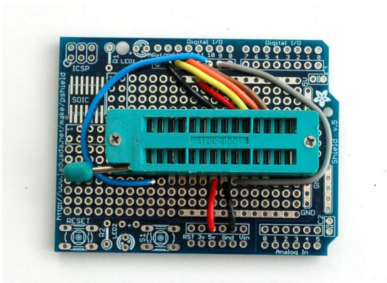
Follow the protoshield tutorial to solder in the Red LED into **LED1** position, Green LED into **LED2** position. Also solder in the two 1.0K resistors next to the LEDs. We'll use the LEDs as
